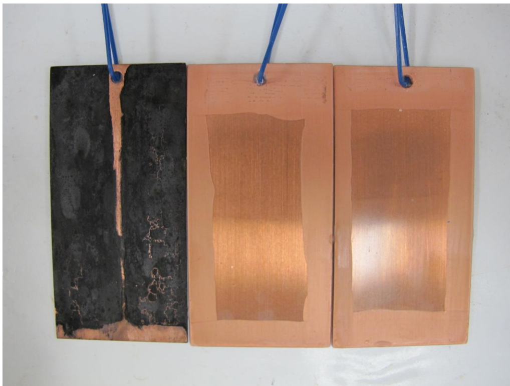
Picture 4: The condition of the copper panels after 1500 hours in the humidity chamber. The control is on the left.
